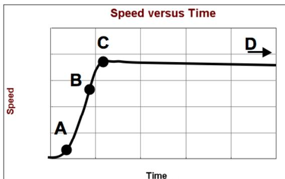
**PART 2.** Your instructor will show you an experiment involving a low-friction cart on a track. The cart will be given a gentle push to start it moving and then, while it is moving along the track, it will be given some more quick taps in the same direction as its motion. Its speed time graph. Measured with a motion sensor, should look similar to this.
