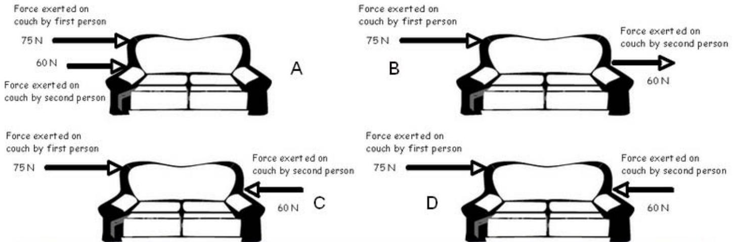
Feedback: Choice B is most appropriate for this situation since it shows a push and a pull of appropriate strengths both acting in the same direction.
