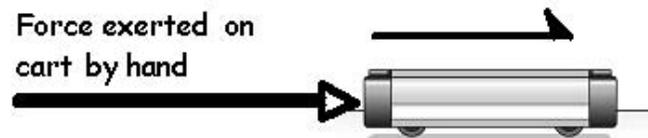
Note that the speed arrow only tells about the speed of the object at the particular moment in time for which the force diagram is being drawn. It does not tell anything about whether the object's speed is in the process of changing, or whether it is remaining constant.
