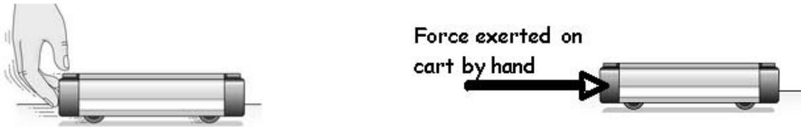
Notice that the force diagram shows only one of the objects involved in the interaction (the cart), and that the other object involved (the hand) is only mentioned in the labeling of the arrow representing the force it is exerting.
