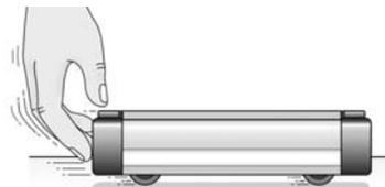
While the cart is moving, and before the data collection stops, give the cart two or three more pushes, in the **same direction** as the first push. (Stop the cart when it reaches the other end of the track.)
