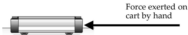
Notice that the force diagram shows only one of the objects involved in the interaction (the cart), and that the other object involved (the hand) is only mentioned in the labeling of the arrow representing the force it is exerting. In this sense these force diagrams are very like the Input/Output (I/O) energy diagrams you drew at the end of Chapter 1.
