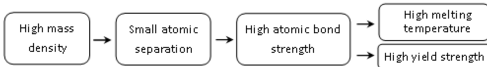
Figure 5.3: Common incorrect line of reasoning about the relation between density, melting temperature, and yield strength. Note that all but one of the steps is incorrect.
