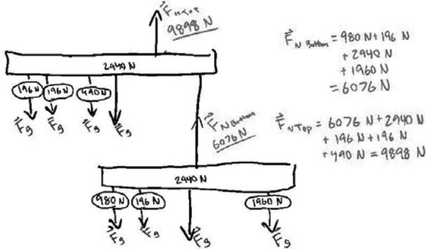
**FIGURE 1.** Example of force diagram.
