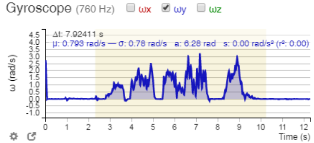
FIG 1. Calibration activity data using the software analysis tools to measure angular displacement.
