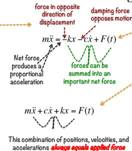
In the initial form, the equation emphasizes the net force as the sum of its parts, which include both a restoring and a damping force, and that the result of this force is to produce an acceleration.
